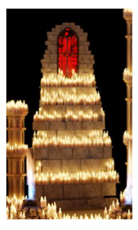
4. 2x Large Pillars - DIMENSIONS; 4000MM x 700mm. Made using polystyrene and a polyurethane coating. Model made in three sections which attach together using box section. Bottom section to have ballast sunk in. Candles sunk into the model and attached with velcro. Design signed off with client. £5,679.55
